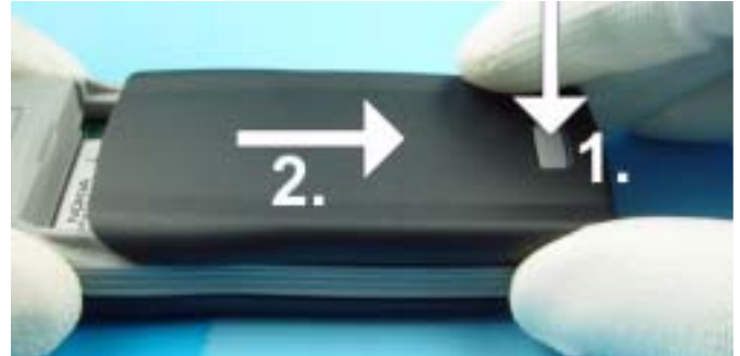
Press the Release Button before removing the Battery Cover.
