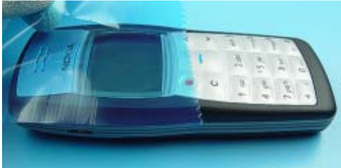
If not already done protect the display window with a film to avoid dust and scratches.
