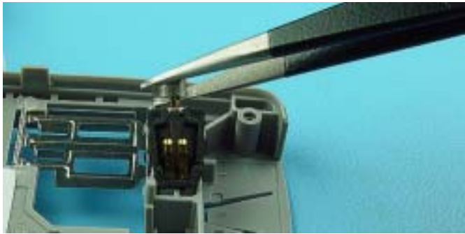
Lever out Vibra Motor with tweezers.
