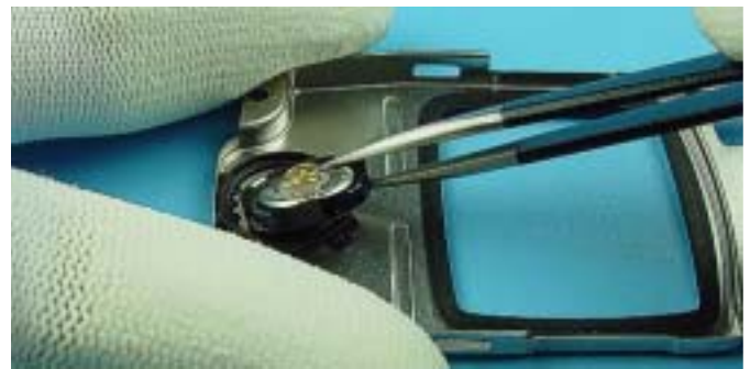
Use tweezers when removing the Speaker.
