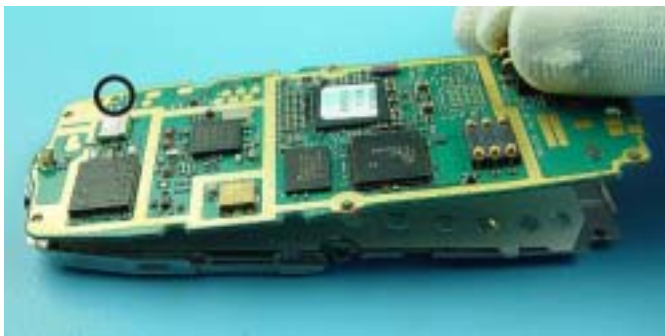
Slowly place Engine Module from top side on.
