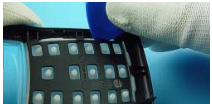
Use SRT-6 to unlock Keymat from A-Cover.
