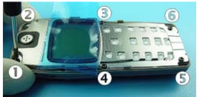
Unscrew the six Torx Plus® size 6 screws. For assembly, the reverse order and a Torx Plus driver with a torque of 21Ncm have to be used.
