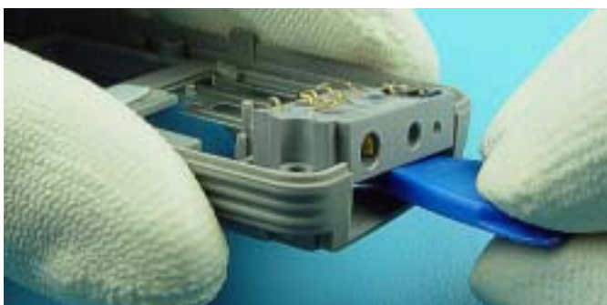
If System Connector is tight in the D-Cover, SRT-6 should be used to loosen it.
