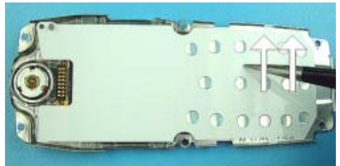
Position Domesheet in direction to the upper right corner, as close as possible to the shielding edge.
