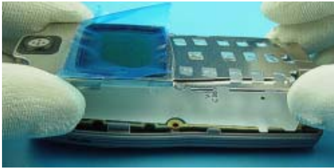
Remove C-Cover from Engine Module.
