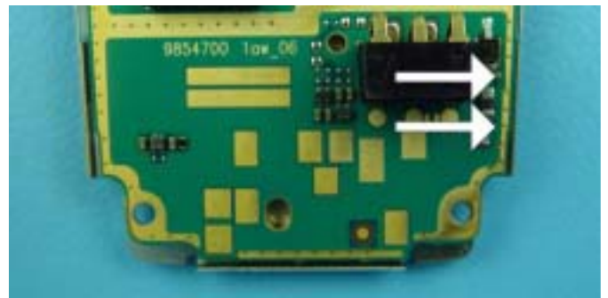
Before sinking the Engine Module, make sure that it is also close to the same side of the shielding.
