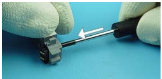
Carefully push out Microphone from System Connector. Moderate force is required for this action.
