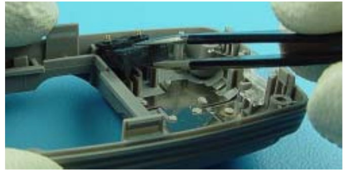
Remove Buzzer from its guidance. Take care not to damage the spring contacts.
