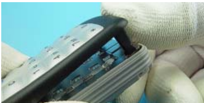
Open A-Cover from bottom side on.
