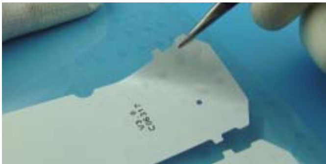
Take a new Domesheet from carrier film. Do not touch the keydomes from lower side.
