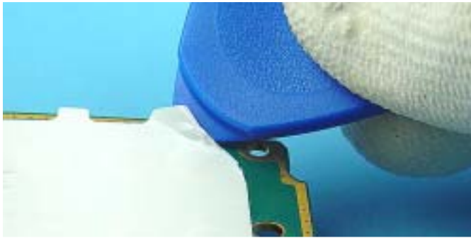
Use SRT-6 to loosen one corner of the Domesheet.
