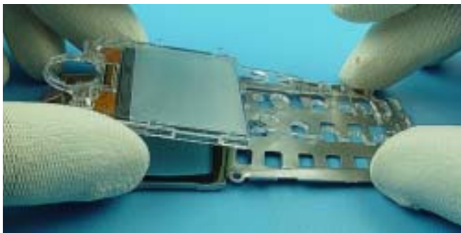
Remove LCD inclusive Lightguide.
