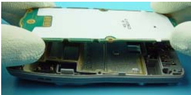
Take Engine Module from D-Cover.
